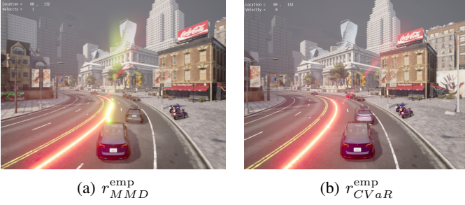
Figure 6: MPC simulations in CARLA. The red line is the route/reference path. Left: trajectory from minimizing r_{MMD}^{emp} . Right: trajectory from minimizing r_{CVaR}^{emp} . With few samples, r_{CVaR}^{emp} varies sharply across MPC steps, often yielding no safe plan (vehicle gets stuck and eventually collides). In contrast, r_{MMD}^{emp} provides a more consistent risk estimate, guiding safe motion.
